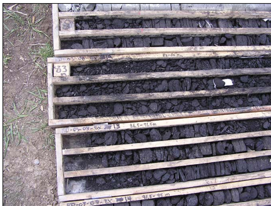
Photo 1: Drillhole BD 08-03, showing the roof contact at 80.3m, and the split core sampling method applied to the initial discovery holes.
