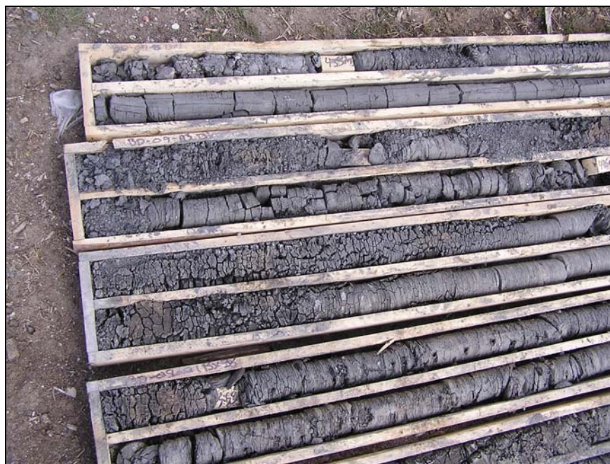
Photo 6: Drillhole BD 09-95, showing slaking mudstones in the upper parts of the hole.
