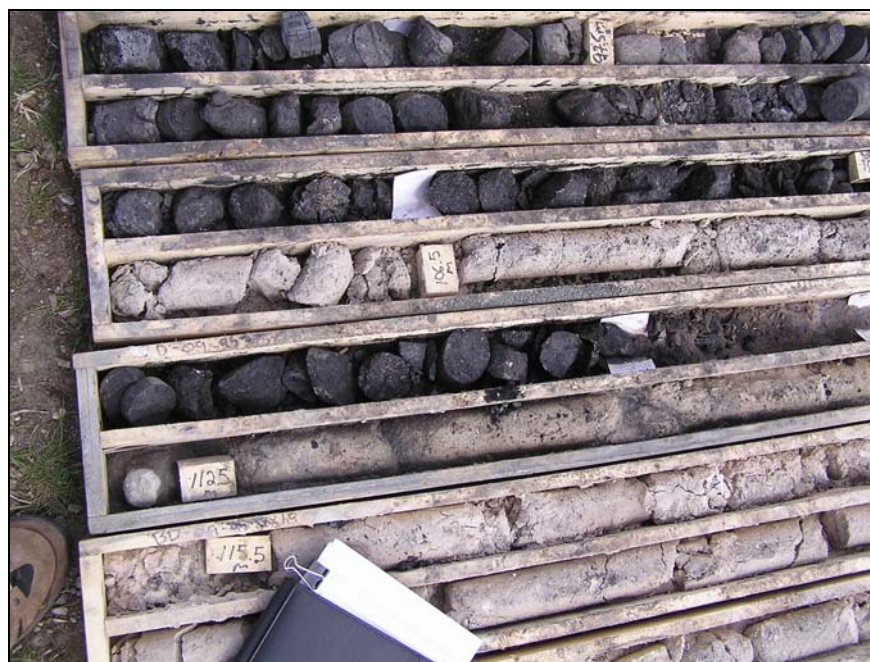
Photo 7: Drillhole BD 09-95, showing the floor contact at 96.12m, the disc and selective whole core sampling method applied to holes during the January-June, 2009 program, as well as the “water sands” (unconsolidated quartz rich sand) below the coal.
