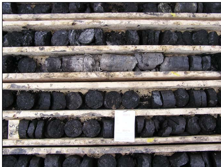
Photo 2: Drillhole BD 09-22, showing a claystone/bentonite parting at 91.49m, and the disc sampling and selective whole core method applied to holes during the January –June 2009 program.
