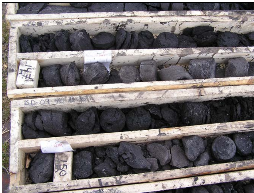
Photo 4: Drillhole BD 09-40, showing several mudstone partings at 147.2m and 150.6m, as well as the disc and selective whole core sampling method applied to holes during the January-June, 2009 program.
