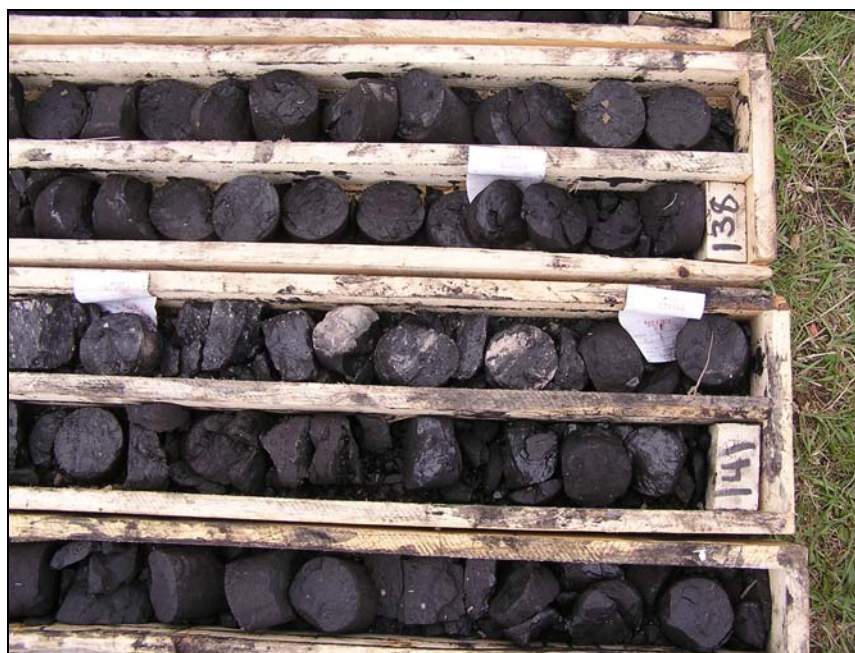
Photo 5: Drillhole BD 09-41, showing fine clay interbeds within the coal, and the sampling method applied to holes during the January – June, 2009 program.
