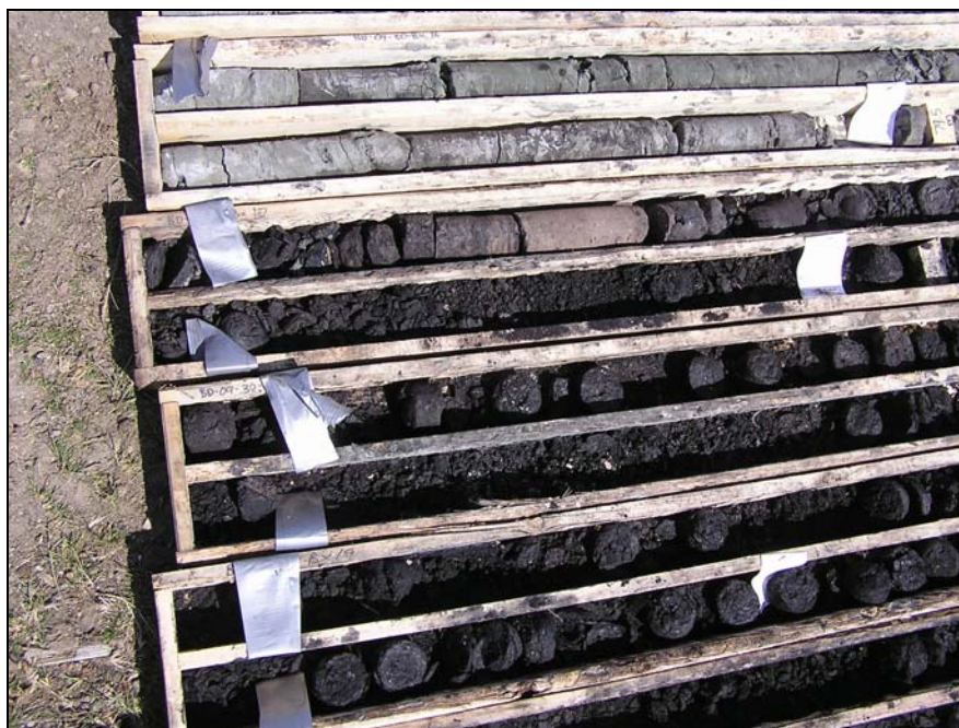
Photo 3: Drillhole BD 09-30, showing the roof contact at 79.8m, and the disc and selective whole core sampling method applied during January –June 2009 program.
